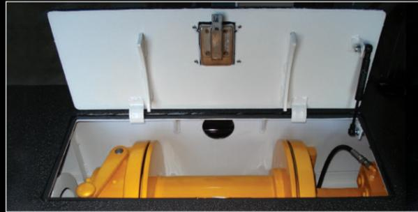
Extra large access door for easy winch operation. Door support and lip seal for maximum strength and less noise.
