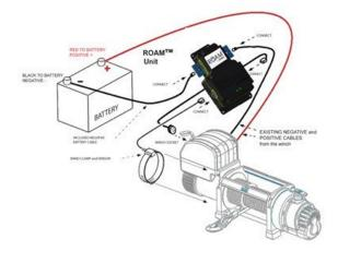
ROAM is hardware and software. The hardware is a logic box that mounts on your vehicle.
