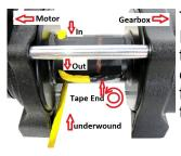
The BC3500 is suited to both steel or synthetic rope. In either installation the rope is fed under the drum from the front of the winch and then into the drum from behind the winch. This is correct with the motor on your left and gearbox on your right when facing the winch. Incorrect rope attachment will not allow the brake to function correctly and support loads..
