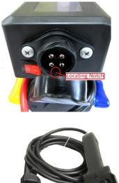
The BC3500 solenoid control box has a 4 pin sock with locating notch. This is used for all plug in control options... The socket is suitable to accept the corded hand held control or the wireless receiver.
