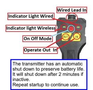
The Wireless transmitter comes paired to the The Wireless transmitter comes paired to the receiver ready for use. Picture shows functions
