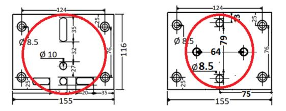
The bolts must be secured with spring washer behind the nut or lock nut should be used. Two flat washers should be used on the bolts on both sides of the mounting plate one under the bolt head and one under the lock washer or lock nut. Ensure all nuts are firmly secured at 30 Nm of torque for M8.
