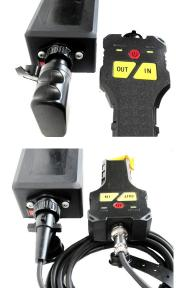
Wireless receiver plugs into the control box
