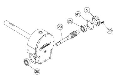
5. Remove bearing cap #5 from gear housing by unscrewing four capscrews #29. Remove worm #23 and bearing #25 from gear housing. Use a soft hammer to gently tap input end of worm and drive worm and bearing from gear housing. Once worm has been removed from housing, bearing can be pressed from end of worm.
