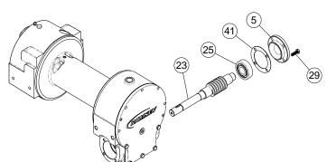
17. Press bearing #25 onto worm and into worm gear housing. NOTE: Be sure thick shoulder of bearing's outer race (side with manufacturer's name and number) is out, away from worm threads. Place gasket #41 onto spur gear housing #15. Secure spur gear housing to worm gear housing using four capscrews #32. Torque capscrews to 7 ft-lbs (9.4 Nm) each.
