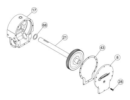
13. Apply grease to end of shaft, opposite gear. Apply grease to bushing in gear housing #17. Place greased end of shaft through thrust washer #68 and bushing in gear housing #17. Place gasket #43 onto gear housing cover #8. Apply grease to gear end of shaft and bushing in cover. Place cover onto shaft and secure to housing with five capscrews #28 at the five lower most holes.
