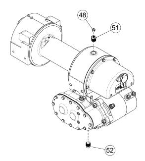
19. Insert plug #52 into bottom of gear housing. Permatex may be applied to threads to help prevent leakage.
