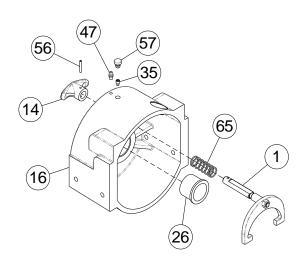
10. Examine shifter assembly #1 for damage to yoke. Yoke should be firmly attached to shaft, yet, able to swivel freely around shaft. Replace if necessary by removing pin #56 from handle #14. Remove rubber plug #57 from housing. Unscrew setscrew enough to allow shifter assembly to be removed from housing.
