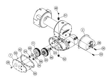
2. Drain oil from spur gear housing by removing #52 plug. Remove cover #7 and gasket #42 from spur gear housing by unscrewing twelve capscrews #28. Slide gear #11 from end of worm shaft. Remove spur gear shaft #20, with gears attached. Check bearings #24 and thrust washers #66 for signs of wear, replace if necessary. Remove old bearing and press new bearings into place.
